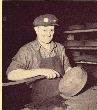
From the core oven the cores are cleaned and assembled for molding and pouring. Ernest Barth uses an air wash on this heater grid core for thorough cleaning.
