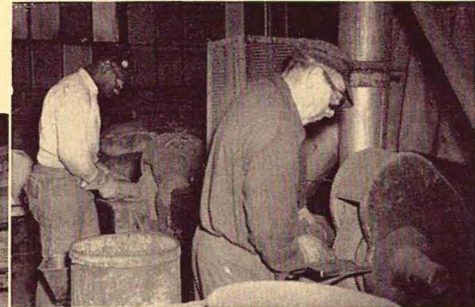
Charles Rose and Rufus Wynns grind gates and fins from "AR" metal castings after Wheelabrator removes all sand and scale.
